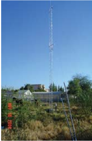
Figure 2.8.2a. A high-resolution data tower that records atmospheric flow and turbulence. This is located at the premises of the Mountain View high school in Mesa, Arizona, and it communicates with a cyber network based at the ASU CLEANER site. In addition to providing data for research, this tower also acts as a facility for high-school student projects. The modus operandi for the ASU CLEANER network is shown in Figure 2.8.2b.
