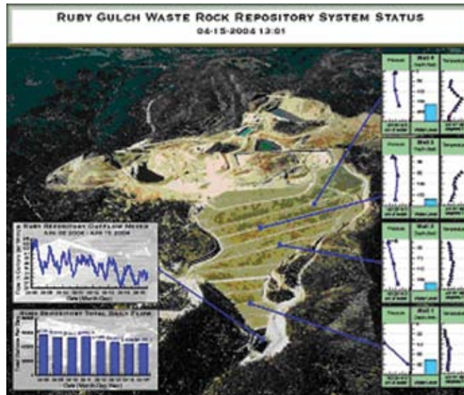
Automatically generated status images of the Gilt Edge monitoring system allow scientists and regulators to compare water data in near real time. (Versteeg et al., 2004)
