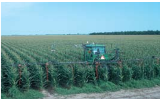
High-clearance vehicle configured with canopy sensors, drop nozzles and controller, which has been designed to deliver liquid N fertilizer based on sensor-determined crop needs.
