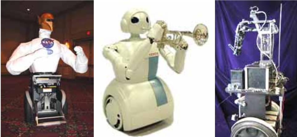
Figure 4.8. Dynamic balancing wheeled humanoids at NASA, Toyota and MIT.
