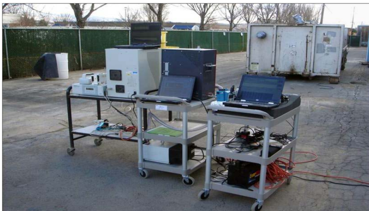
Figure 4.8. Example of field application of instruments needed for real-time measurement of number, mass, size distribution, and surface area of engineered nanomaterials.
