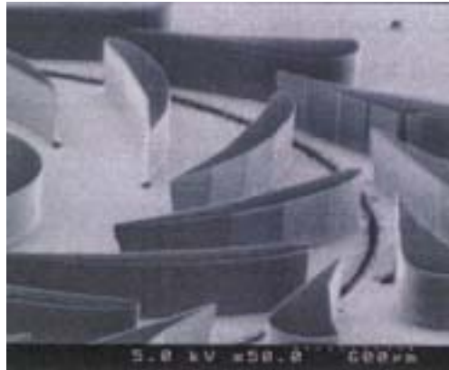
Figure 6.3. Micro air turbine capable of 10,000 rpm. The prototype rotor is 5 mm in diameter and fabricated from SiN ceramics by nitridation of silicon powder (Esashi Lab, Tohoku University).
