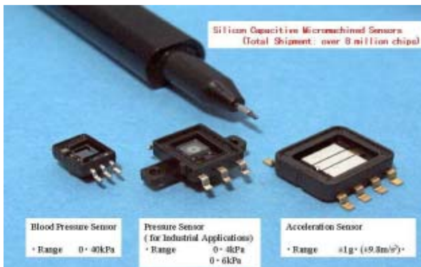
Figure 4.6. The Omron foundry strategy is to augment production demand that is also being used to produce these pressure sensors and accelerometers (Horiike et al. 2001).
